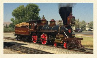
The "Inyo" of the Virginia and Truckee Railroad is a 2'B steam locomotive built in 1875 by the Baldwin Locomotive Works. It was used for both passenger and freight service. In 1877, it was equipped with air brakes and converted from wood to oil firing in 1910.
